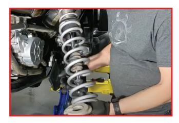
Install new rear billet cross over ring. Loosen the allen screws with a 3/32" allen wrench. Do not loosen allen screws all the way out.
