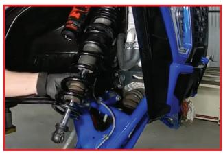
Install lower OEM spring retainer by reconnecting lower shock bolt to a-arm. Push down and hold a-arm to fully extend internal bump stop spring.
