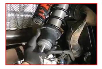
Install new main spring and OEM lower spring retainer.
