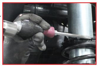
Rotate OEM preload rings counter clockwise all the way to top of threaded shock body. OEM spring stack is now loose.
