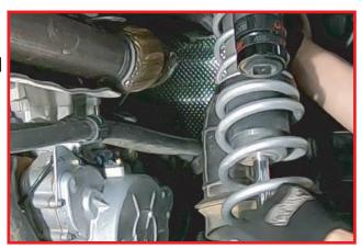
Disconnect lower shock bolt from trailing arm. Swing lower shock rearward and out.
