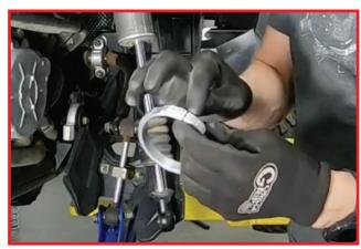
Starting at the bottom of the threaded shock body, rotate the cross over ring counter clockwise up the threaded shock body. Be careful not to cross thread and damage cross over ring or threaded shock body. Set cross over ring 6" from shock body cap. Do not tighten cross over ring, it will need to be moved once preload is set.
